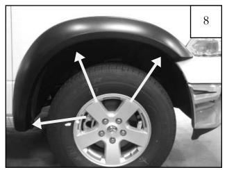
Hold flare to the vehicle and start additional supplied screws with a Phillips Head Screwdriver through the factory holes. *Do not tighten*.
